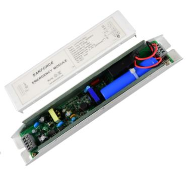
LCP013C002L: O/p Power=2 W, Illumination Time=3 Hours LCP012C003L: O/p Power=3 W, Illumination Time=2 Hours LCP012C004L: O/p Power=4 W, Illumination Time=1.5 Hours
